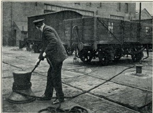
This man is obviously standing in the wrong position as the capstan rope when tightened is likely to cause injury.
